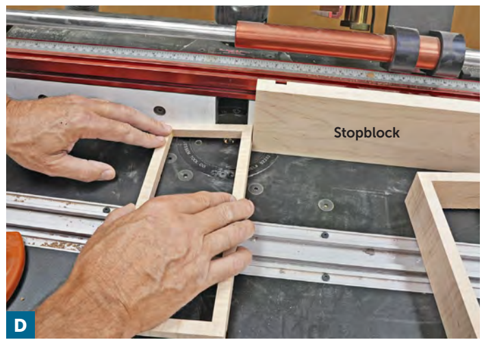
D Reposition the stopblock to the other side of the bit for the remaining mortises. Set the top (and base) against the stopblock and lower it onto the spinning bit, then pull the workpiece along the fence.
