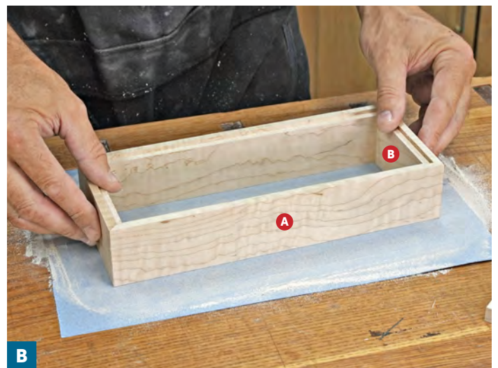
Attach 150-grit sandpaper to a flat surface. Remove any blade or burn marks on the mating edges of the box top and base by sanding in small, circular motions.
